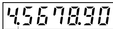
Power save mark (Mark only lights up in the power save mode.)
